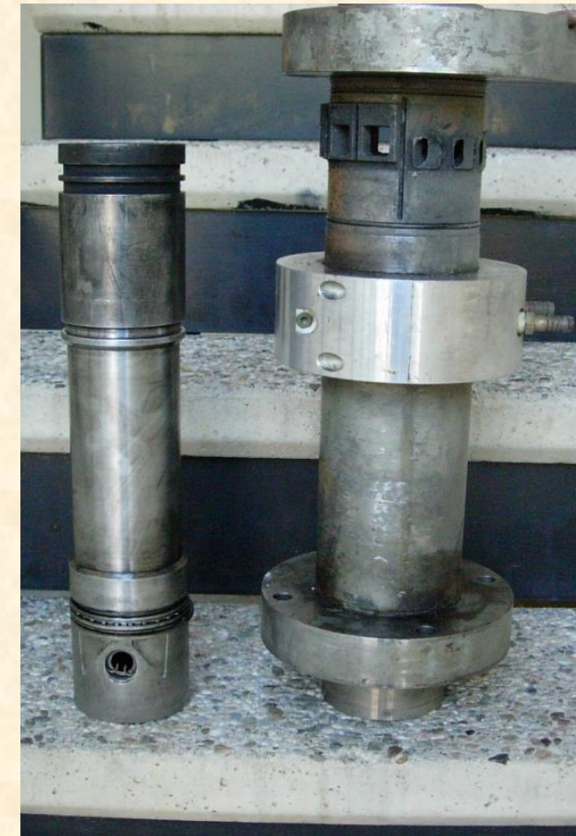
DETAILS OF THE ELONGATED CYLINDER-PISTON ASSEMBLY SHOWING THE POSITION OF THE WINDOWS
