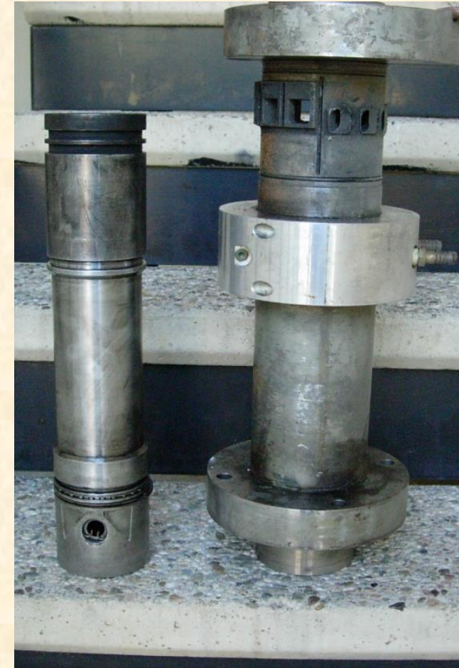
DETAILS OF THE ELONGATED CYLINDER-PISTON ASSEMBLY SHOWING THE POSITION OF THE WINDOWS
