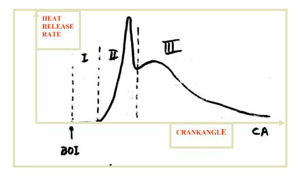
Figure 1. Three phases of the combustion in a direct-injected diesel engine. I. IGNITION DELAY PERIOD, II. PREMIXED COMBUSTION PHASE, III. MIXING-CONTROLLED COMBUSTION.
