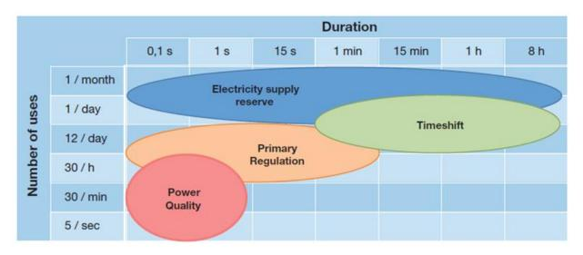
Figure 1.3. Different uses of electrical energy storage in grids, depending on the frequency and duration of use.
