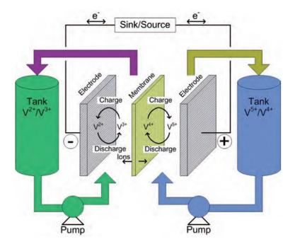
Figure 2.7. Schematic of Vanadium Redox Floe Battery
