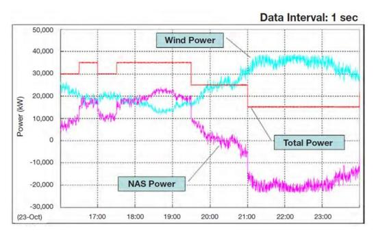
Figure 3.11. Example operational results of constant output control over 8 hours (NGK)
