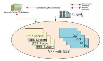
Figure 3.19. A generalized control concept for aggregated energy systems and DGs
