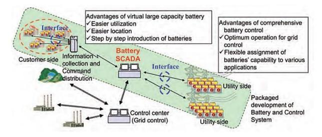
Figure 3.20. Schematic diagram of battery SCADA.
