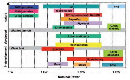
Figure 2.11. Maturity and state of the art of storage systems for electrical energy
