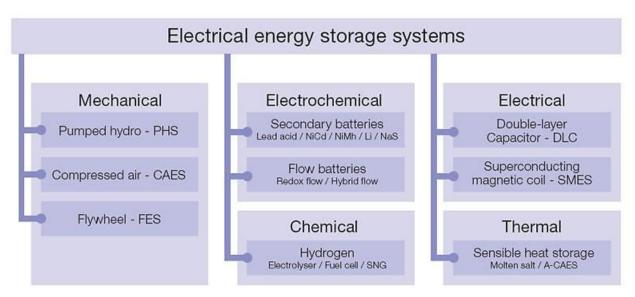
Figure 2.1. Classification of electrical energy storage systems according to energy form
