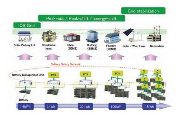
Figure 3.13. Scalable architecture for energy storage applications in a smart microgrid (Sanyo)
