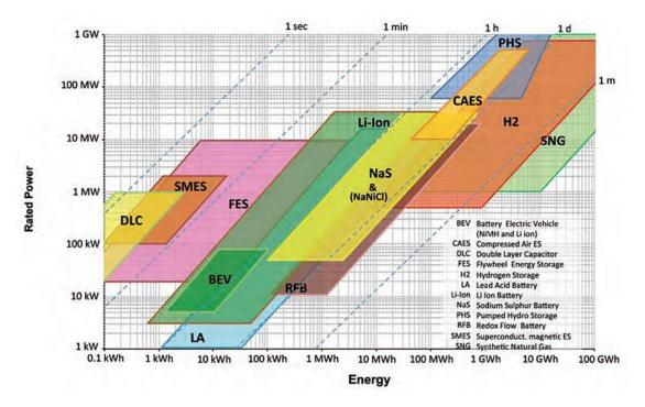
Figure 2.9. Comparison of rated power, energy content and discharge time of different energy storage technologies
