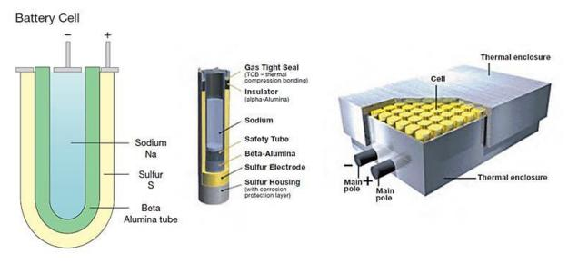
Figure 2.6. NAS Battery cell design and 50 kW module (NGK)
