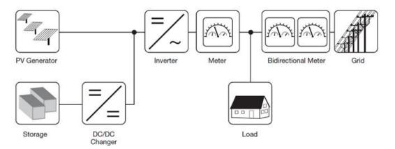
Figure 3.7. Photovoltaic system designed for energy self-consumption
