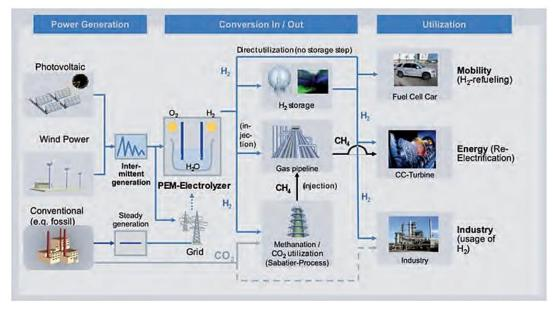
Figure 2.8. Overall concept for the use of hydrogen and SNG as energy carriers
