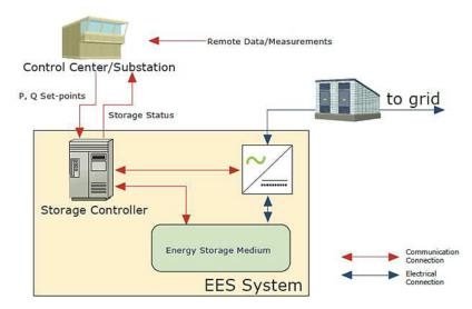
Figure 3.18. A Control hierarchy involving remote data/measurements (ABB)
