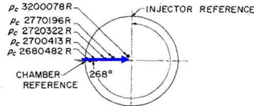
Pressure distribution across the injector radius vs time during resonant combustion – Standard chamber. These records obtained ~25 ms from bomb pulse
