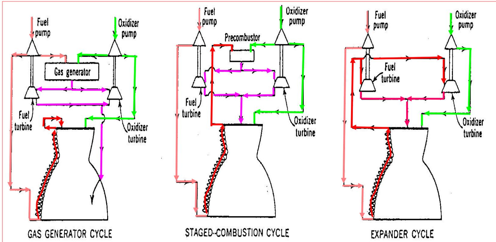
**Different engine cycles used for liquid rocket engines**
