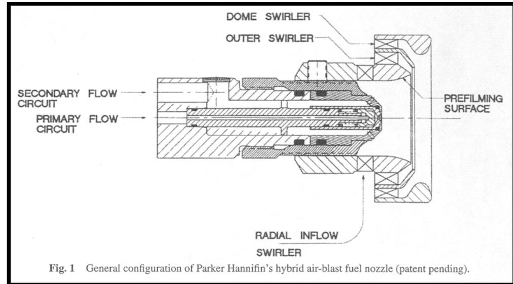
**Hybrid airblast fuel injector**
