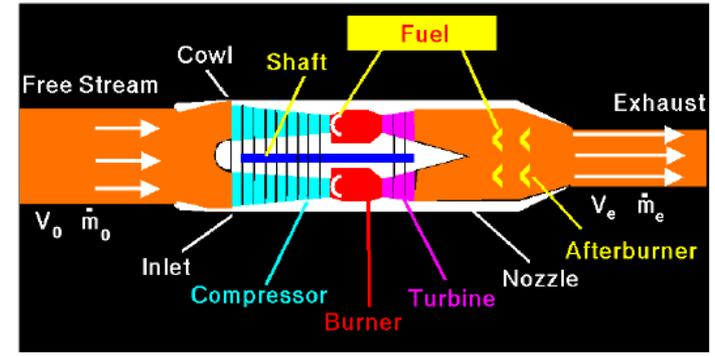
$$\text{Thrust} = F = \dot{m}_e V_e - \dot{m}_0 V_0$$
