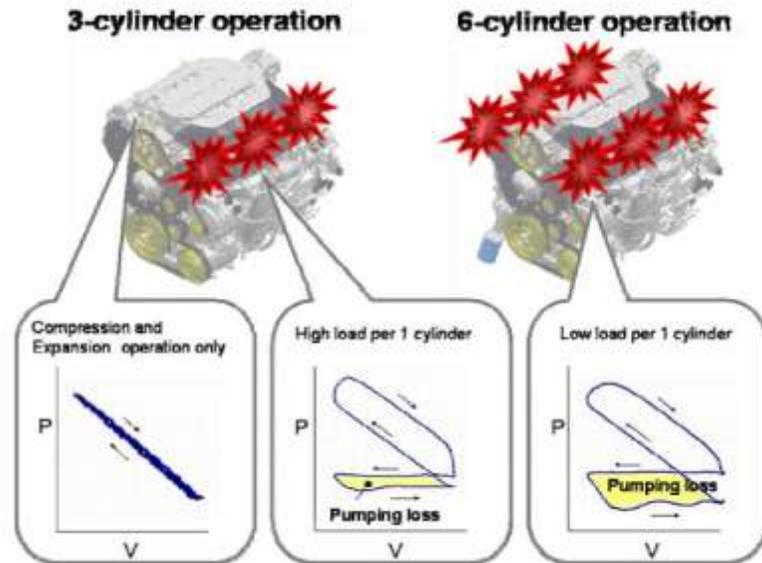
There is also the all-new 2016 Honda Pilot SUV with 3.5 L, Gasoline Direct Injection (GDI) i-VTEC, 11.5 CR, V6 engine with new two-stage VCM technology. For further fuel saving, this engine also includes a *stop-start feature*. This appears to be Honda's first non-hybrid application of this technology.
