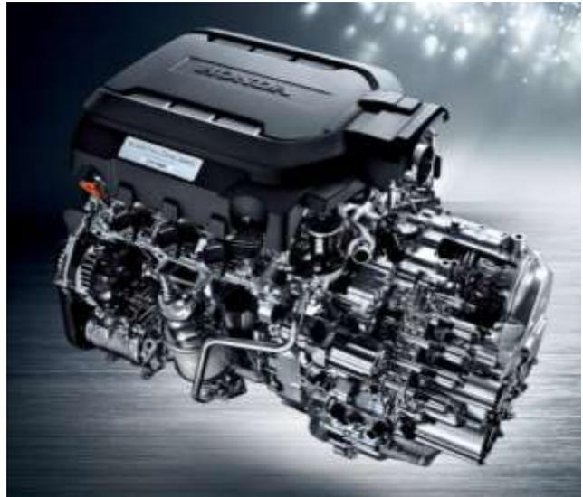
*i-VTEC with 3-stage VCM.* The basic idea is that the vehicle only requires a fraction of its power output at cruising speeds. The system electronically deactivates cylinders to reduce fuel consumption. This engine is able to run on 3, 4, or all 6 cylinders based on the power requirement. One receives V6 power when accelerating or climbing hills as well as the efficiency of a smaller engine when under cruising condition.
