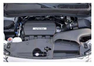
In Honda's VCM V-6, the hydraulic circuit consists of two systems, each capable of providing the pressure needed to actuate the synchronizing piston that disables the unneeded valves. This is accomplished by separating the two tandem rocker arms that work with each valve, causing it to remain shut.
