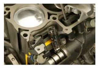
selected valves in this overhead-valve design.Switching between 8- and 4-cylinder operation could take place in 40 milliseconds, according to Chrysler, and no fuel entered the unused cylinders. Chrysler claimed a fuel-economy improvement of 10 to 20 percent for Multi-Displacement in this Hemi V-8 engine.
