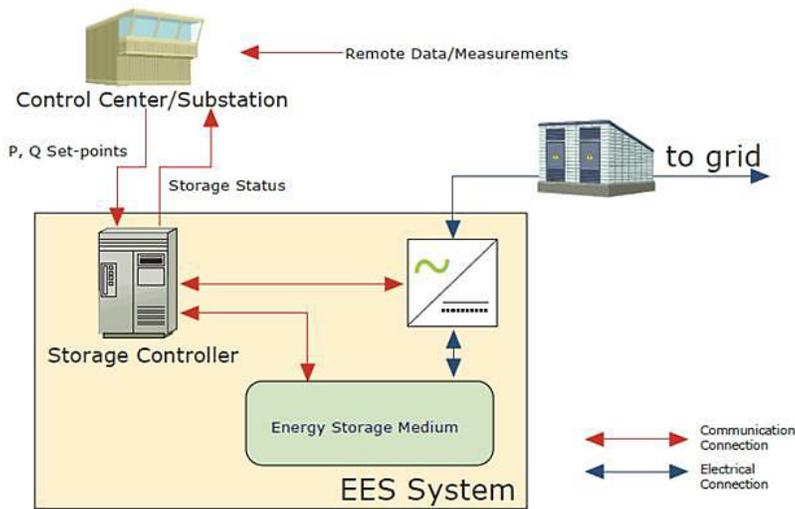
Figure 3.18. A Control hierarchy involving remote data/measurements (ABB)
