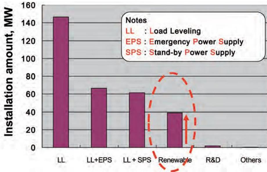
Figure 3.4. NAS Battery applications and installed capacities
