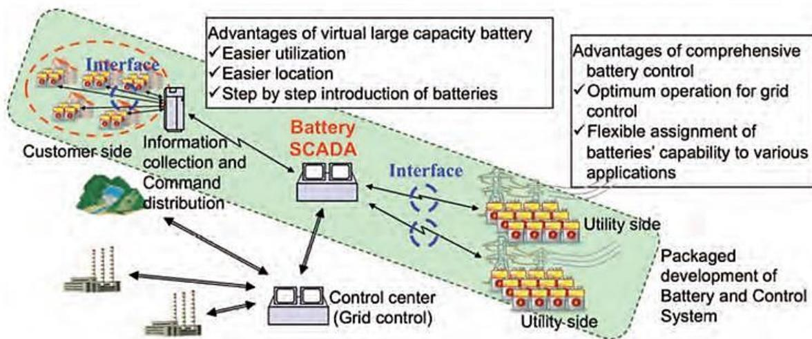
Figure 3.20. Schematic diagram of battery SCADA.
