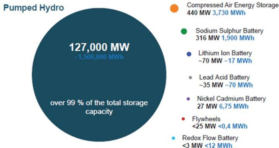
Figure 3.6. Worldwide installed storage capacity for electrical energy
