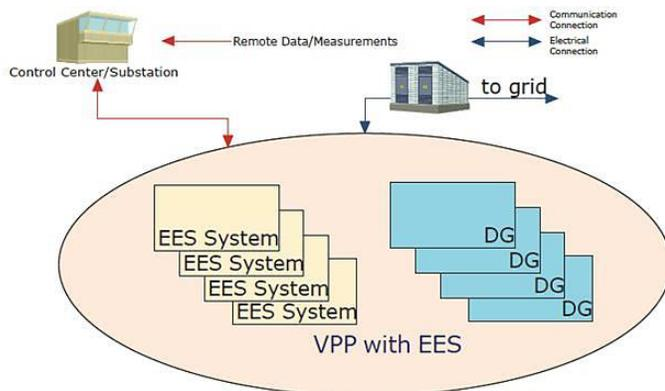
Figure 3.19. A generalized control concept for aggregated energy systems and DGs
