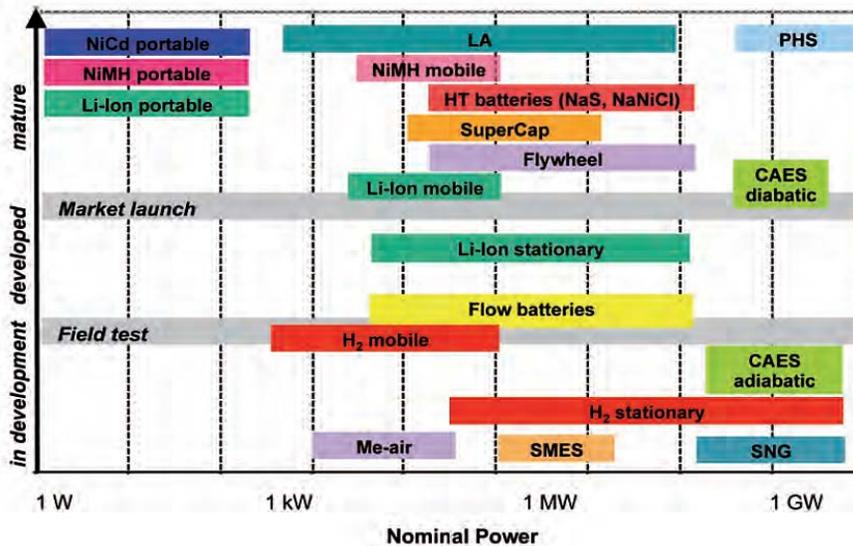
Figure 2.11. Maturity and state of the art of storage systems for electrical energy
