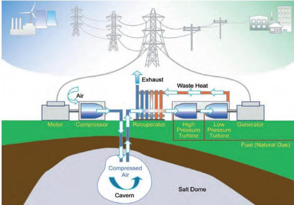
Figure 2.3. Underground compressed air energy storage (CAES).
