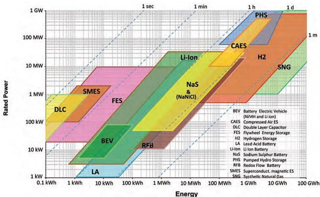
Figure 2.9. Comparison of rated power, energy content and discharge time of different energy storage technologies
