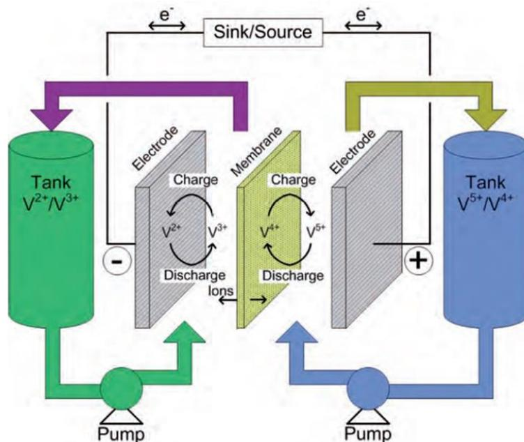
Figure 2.7. Schematic of Vanadium Redox Flow Battery
