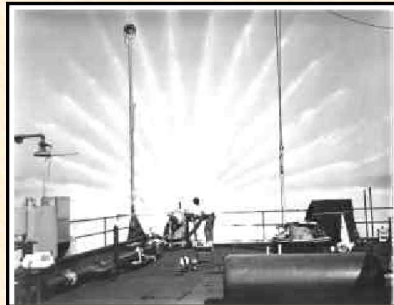
Water flow test of pintle injector for Air Force 250,000 lbf Engine
